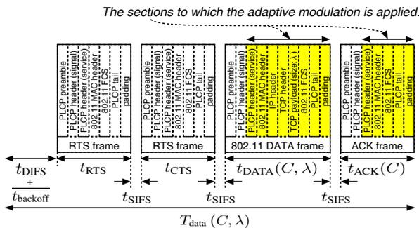
Fig. 2. Calculation of  $T_{\text{data}}(C, \lambda)$  (in case of IEEE 802.11a)
