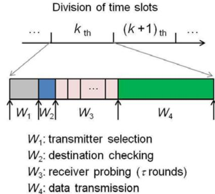
Fig. 2. Partition of a time slot.
