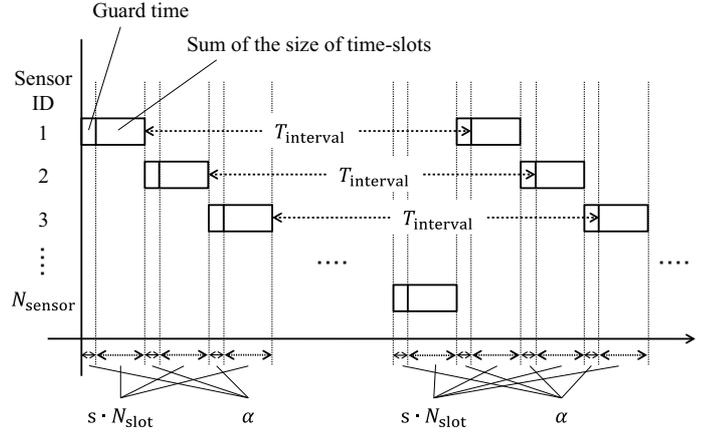
Fig. 2. An example of TDMA based on the fixed size time-slot.
