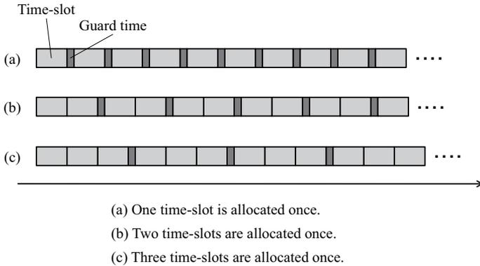
Fig. 3. Different time-slots allocation methods.
