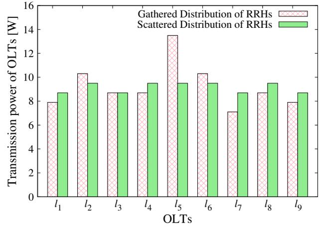
Fig. 4. The transmission power of OLTs in the GDR and SDR.
