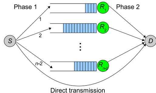
Fig. 1. Illustration of the two-hop relay routing protocol, where the destination node  $D$  receives a packet either directly from the source node  $S$  or from one of the  $n - 2$  distinct relay nodes.
