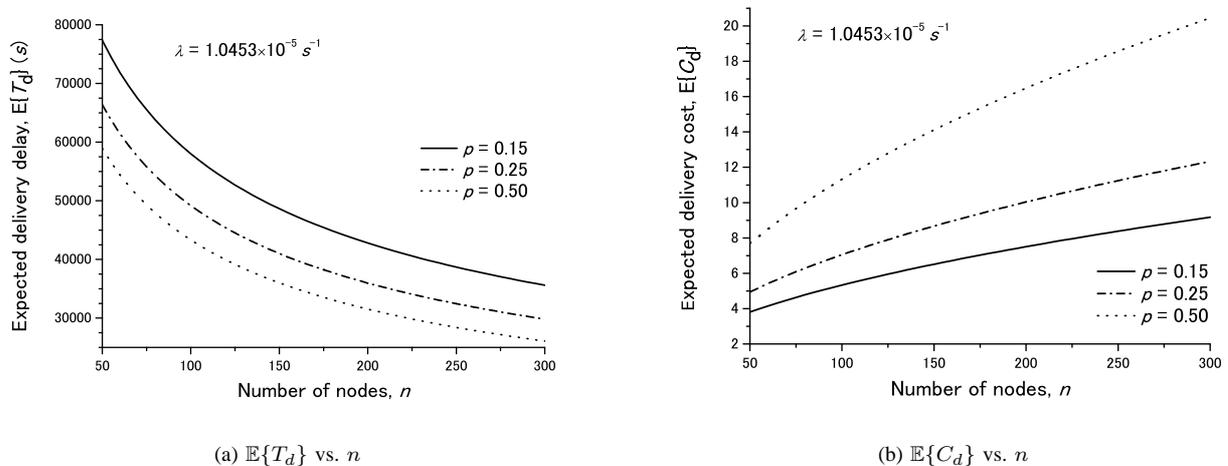
Fig. 5. The expected delivery delay  $\mathbb{E}\{T_d\}$  and expected delivery cost  $\mathbb{E}\{C_d\}$  vs. the number of nodes  $n$ .
