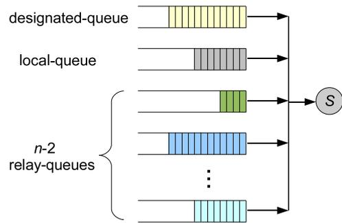
Fig. 2. Illustration of the queue structure at the buffer of node  $S$ , which contains one designated-queue for packets destined for itself, one local-queue for its locally generated traffic and  $n - 2$  parallel relay-queues for traffic of other flows.
