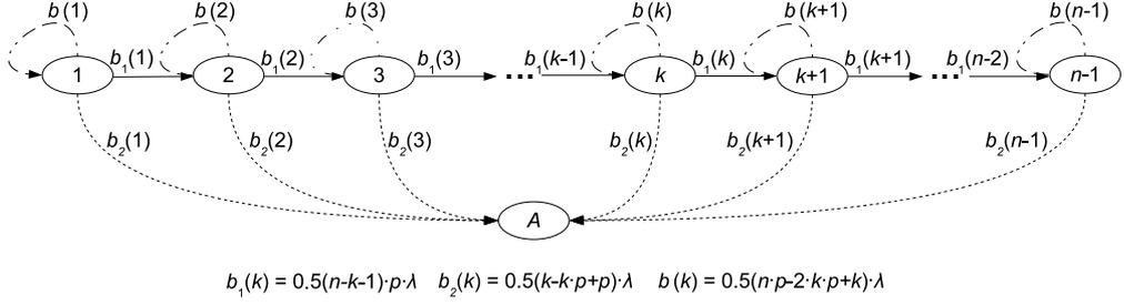
Fig. 3. Transition diagram of the finite-state absorbing CTMC for the HoL packet  $P_h$  of the local-queue at the source node  $S$ , given that the destination node  $D$  is also requesting  $P_h$ . For each transient state  $k$ , the corresponding transition rate  $b_1(k)$  to its neighboring state, the transition rate  $b_2(k)$  to the absorbing state  $A$  and the transition rate  $b(k)$  to itself are listed at the bottom part of the figure.
