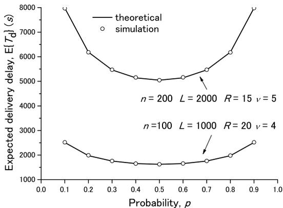
(a) Theoretical and simulation  $\mathbb{E}\{T_d\}$  vs.  $p$
