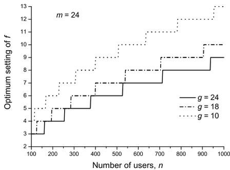
(b) Optimum setting of  $f$  vs.  $n$ Fig. 9. Optimum parameter settings vs. number of nodes  $n$
