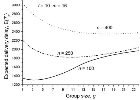
(a)  $\mathbb{E}\{T_p\}$  vs.  $g$
