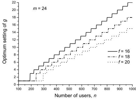
(a) Optimum setting of  $g$  vs.  $n$
