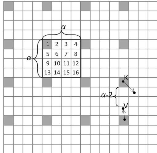
Fig. 3. An example of a concurrent-set of cells with  $\alpha = 4$ . The cells are divided into 16 different concurrent-sets and all the shaded cells belong to the same concurrent-set. The distribution of all the remaining nodes in the unit square is not shown for simplicity.
