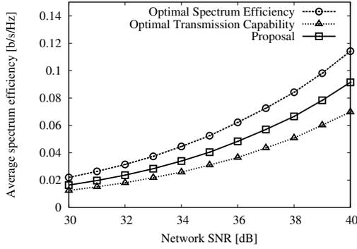
Fig. 7. Average spectrum efficiency of the network ( $\mathfrak{R}_G$ ) with different values of network SNR.
