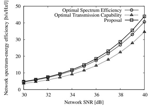
Fig. 9. Network spectrum-energy efficiency ( $\Omega_G$ ) with different values of network SNR.
