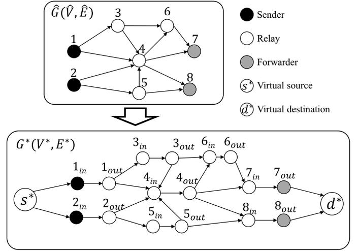
Fig. 3. Transforming the topology  $\hat{G}(\hat{V}, \hat{E})$  to an extended graph  $G^*(V^*, E^*)$ . Every node  $v$  in  $\hat{G}$  is transformed to two nodes,  $v_{in}$  and  $v_{out}$ , in  $G^*$ . A virtual source  $s^*$  and a virtual destination  $d^*$  are added to  $G^*$ .
