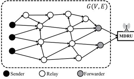
Fig. 2. The categories of nodes in the network  $G(V, E)$ . In the real network, the forwarders are the gateways that have direct connections with the MDRU in the routing paths.
