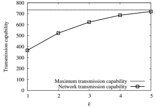
Fig. 5. Transmission capability of the network ( $\Gamma_G$ ) with different values of  $k$ .
