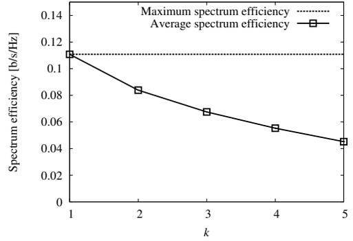
Fig. 4. Average spectrum efficiency of the network ( $\mathfrak{R}_G$ ) with different values of  $k$ .
