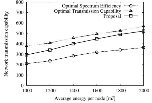
Fig. 8. Transmission capability of the network ( $\Gamma_G$ ) with different values of the average energy per node.
